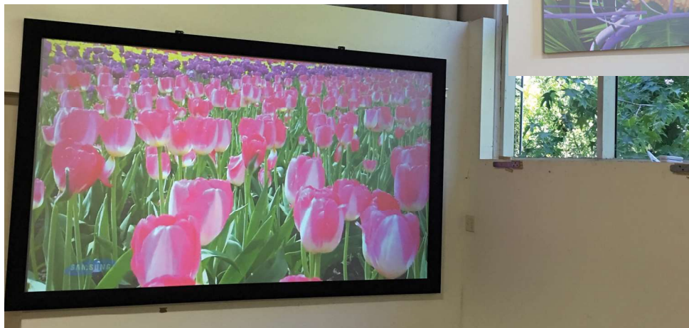
Above: Undoctored photo of ambient light from an outside source washing out a matte white projection screen. Left: undoctored photo of an ALR (Ambient Light Rejecting) screen.
